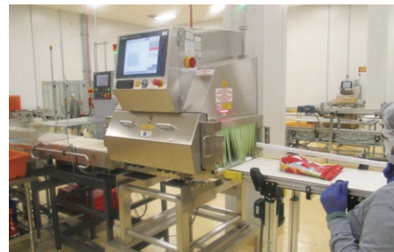
X-ray inspection in Morinaga America Foods, Inc.
